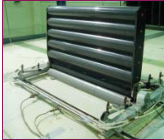
Model of OYSTER in the wave-tank at QUB
