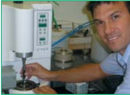
Resistance of the asphalt mixtures to damage in dry/wet conditions assessed by means of a Dynamic Mechanical Analyzer (DMA)
