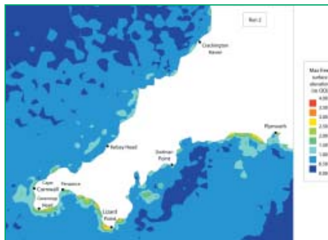
"Worst-case" water elevations around the Cornish coast following an Atlantic tsunami are predicted generally to be less than those already anticipated in the design of coastal defences.
