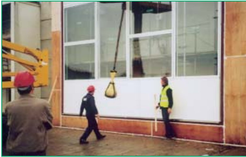
Impact testing of a curtain wall
