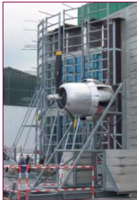
Facade watertightness testing: dynamic aero engine method in accordance with CWCT 'Standard for systemised building envelopes', courtesy Wintech.
