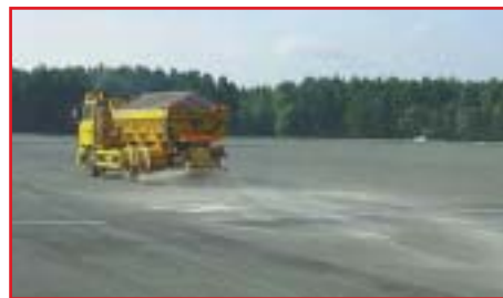
Spreader discharging salt onto the road surface during tests
